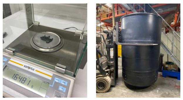
Melt index measurement and a rotation moulded recycled plastics test well of MolokClassic.
